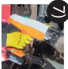
Apply Marker flat to part and hold firmly in place. For smaller or odd parts, adjust wing-nuts on head so marking pin tip is a few mm from Cat part surface. Press Trigger. Once to align pin to starting point, & 2nd trigger pull to begin marking!
